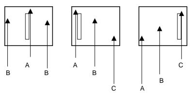
Point A will have best efficiency; Point B will have normal efficiency; Point C will have less efficiency
